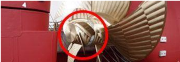
MOL Developed PBCF Reduces 3-5% Fuel Consumption
